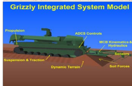
c) Integrated System Model with automatic depth control and calibrated soil mechanics
